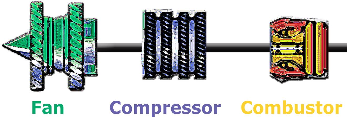
The **FAN** blades spin at high speed (because of air rushing in) and **COMPRESS** or squeeze the air in the compressor.
